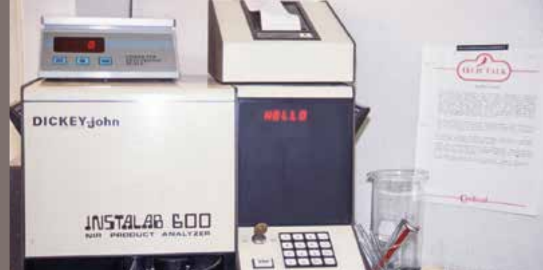
Images left to right: (1) Cardinal's original near infrared fat analysis equipment. (2) The original DNA testing equipment used by Cardinal.
