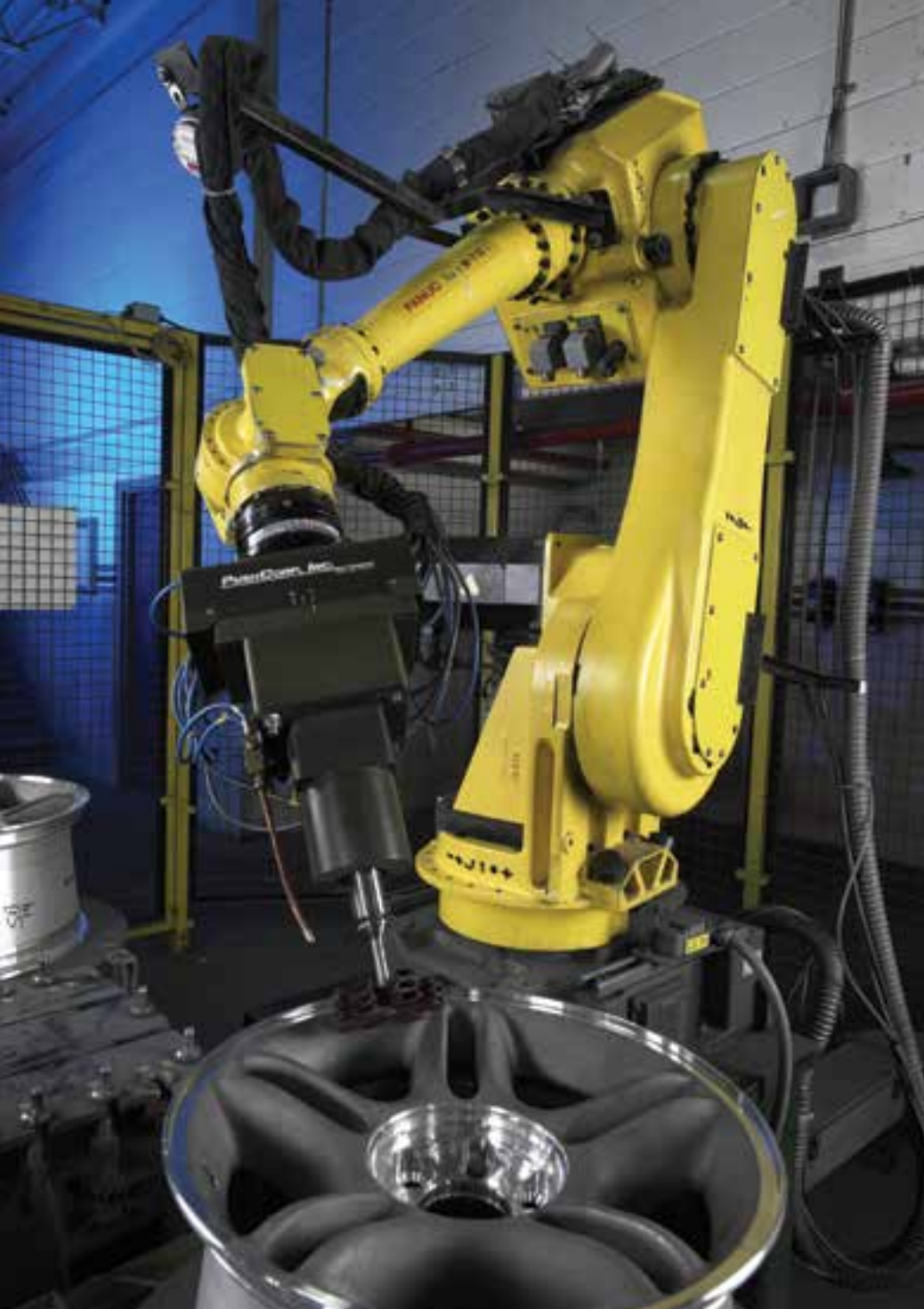
Developmental cell used for initial program for robotic polishing.
