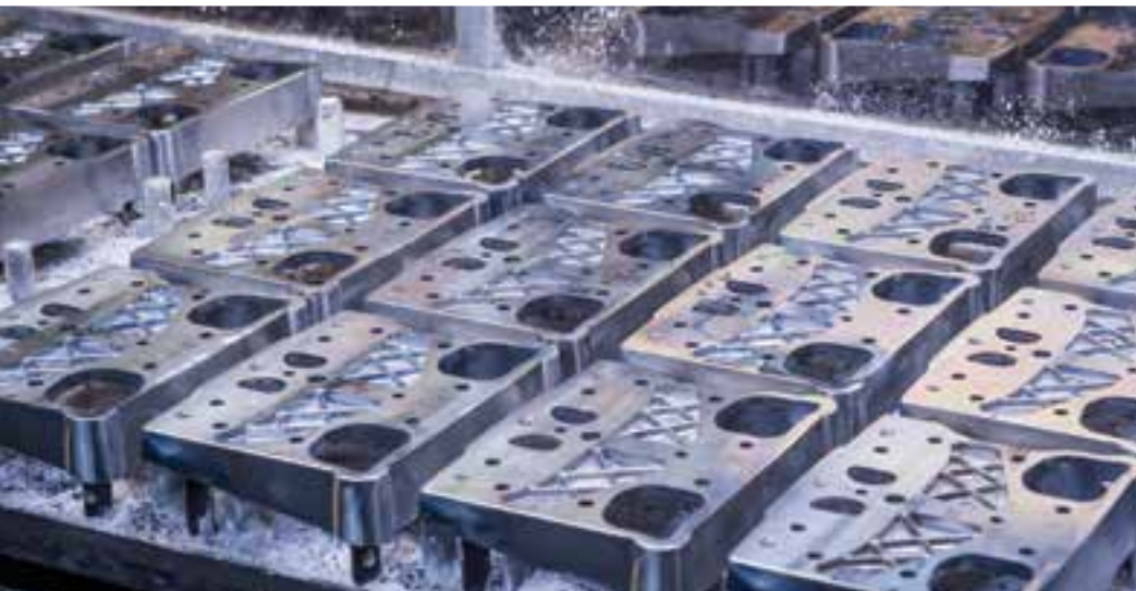
Housings about to go into a robotic polishing cell.
