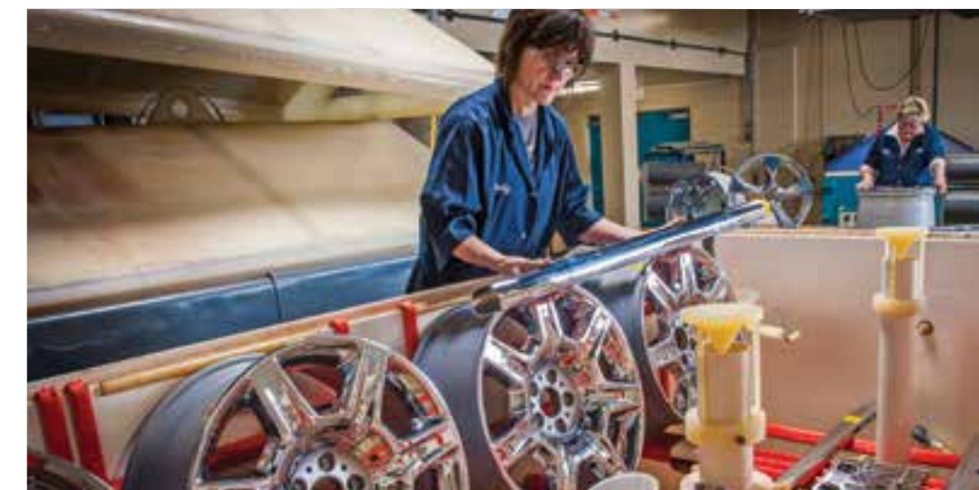
Charlene Sheen-Jauch working at the CASS cabinet to perform CASS tests on wheel parts with Betty Germann in the background.
