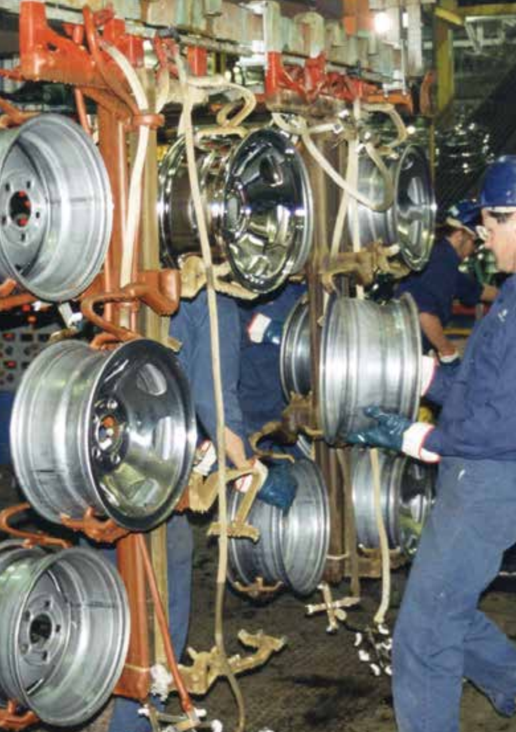
Racks with aluminum wheels going into the plating tank at the Hoist Aluminum line.
