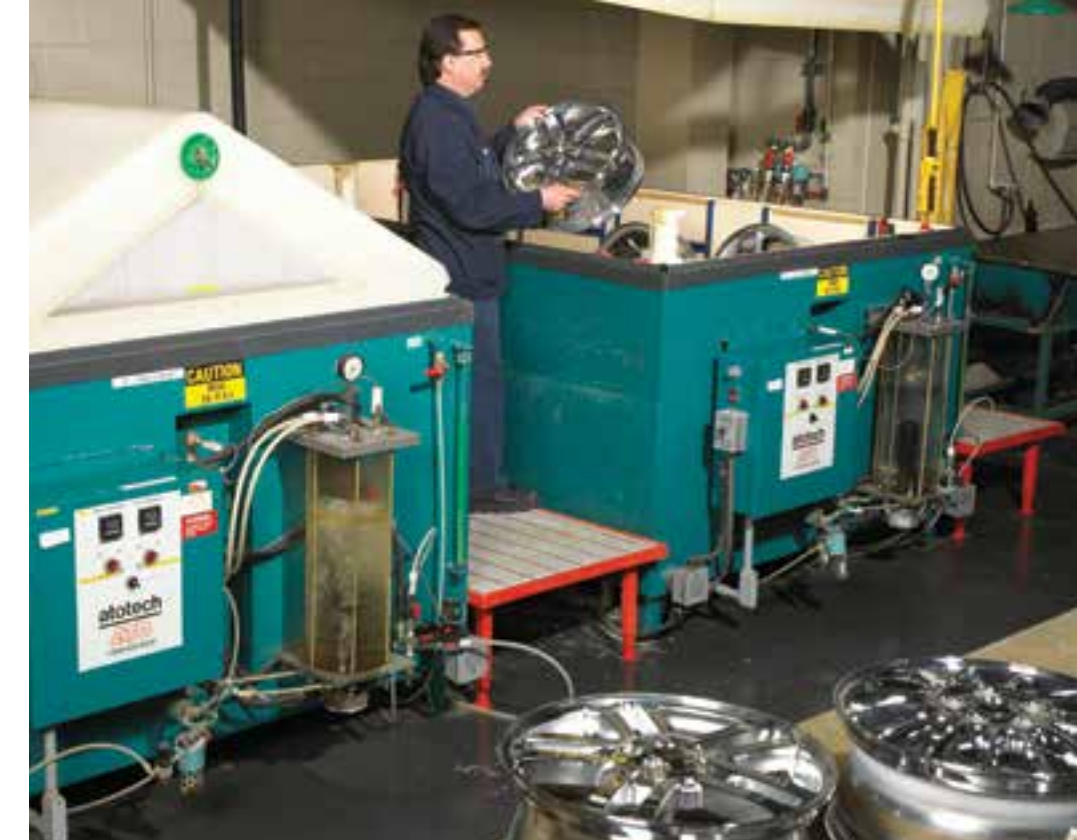
Mike Ball at the custom-made CASS cabinets used for CASS testing in the QC lab.
