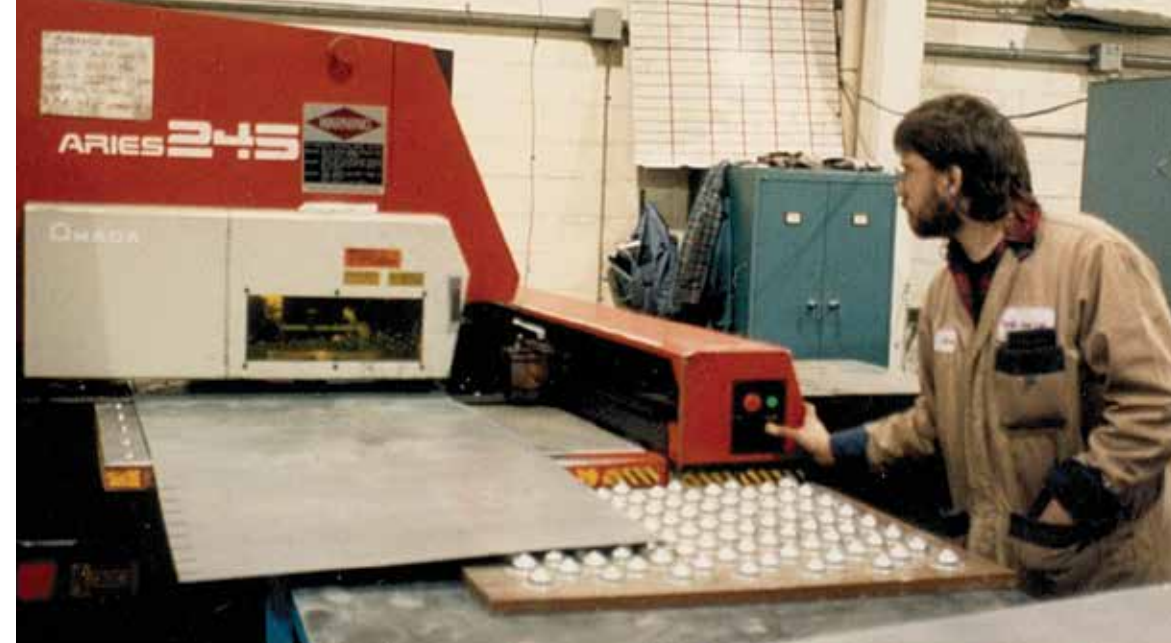
First CNC punch press used in the production of fireplaces, late 1980's.
